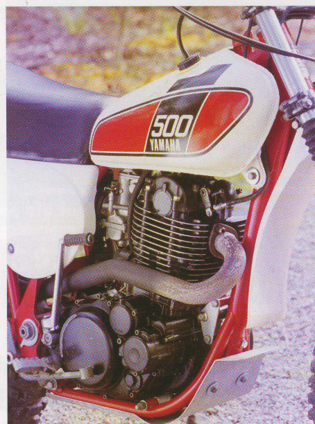
Engine installation required no fabrication or special fittings
